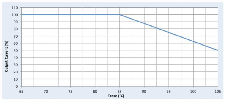
Note: There is ±5°C tolerance on the driver case temperature
